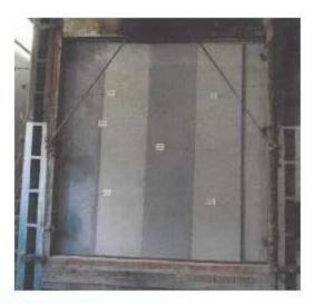
On the left picture; SABS burns one side of the panels for one hour at 1000 degree. The opposite side of the wall was intact and not overheated.
