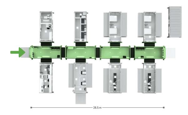
The entrance section of the field hospital is designed to connect different departments together and create a modular space. Made up of 4 containers, this corridor also houses essential electrical and ventilation systems, ensuring the hospital is fully functional. With this modular design, more departments and patient beds can be easily added as needed, based on customer requests.
