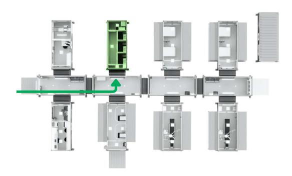
This container boasts a dual functionality, serving two distinct purposes. While one section of the container is designated as a restroom area, the remaining space at the back is specifically designed to function as a laundry area. The laundry area is intended to facilitate the washing and drying of materials used in field hospitals, ultimately leading to their sterilization. Three toilet cabins have been placed by utilizing the space in the most efficient way.
