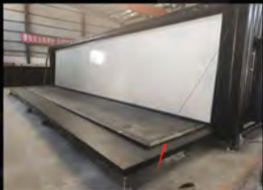
Stainless steel sliding rails + water-stop frame
