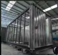
Reinforced structure with galvanized square pipes
