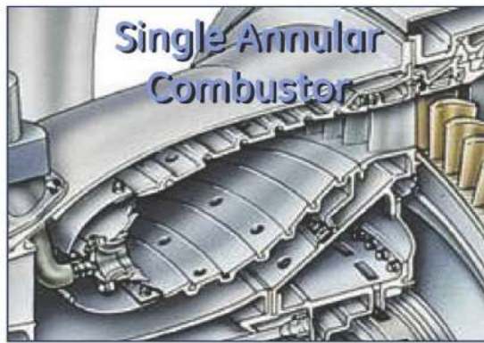
Figure 32: Single annular combustor vs Triple annular combustor
